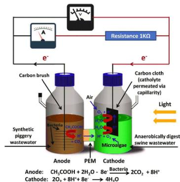
Fig. 2: Energy neutral wastewater treatment via microbial fuel cells.
